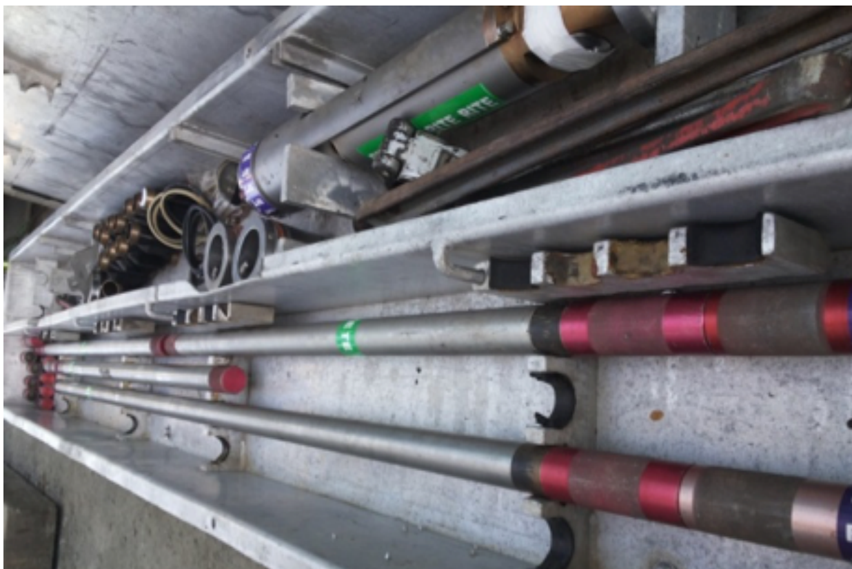
Figura 2 – Conjunto de MWD ( Measurement While Drilling ).
